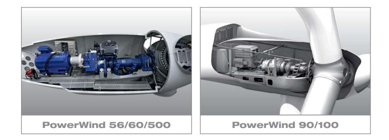
The PowerWind 56/60 is a state-of-the-art wind turbine, certified<br/>under IEC wind class IIA/IIIA and DIBt WZ III/II. It has a rated power of<br/>900/850 kW and a rotor with a diameter of 56/60 m.The PowerWind 90/100 is a highly efficient 2.5-MW wind turbine. It has<br/>a 90/100 m rotor diameter. Certified under IEC wind class IIA/IIIA, it is<br/>ideal for use at locations with medium to high wind speeds.
